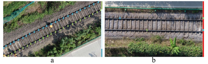
FIGURE 2. Illustration of the traditional "vertical sampling and horizontal positioning" row anchor-based method (Qin et al., 2020), in which an image is gridded into many cells and an extra cell is attached to the end of each row of cells indicating no railway track exists in that row. (a) shows a normal case with this representation method. (b) shows a typical failure case under this formulation.
